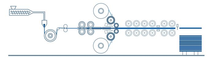
EconCore licenses technologies for continuous production of honeycomb sandwich panels. Excellent cost positon of the product is achieved thanks to the fully integrated manufacturing process but also due to the fact that the honeycomb sandwich design allows to minimize the amount of otherwise expensive materials.
