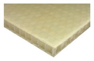
Integration of the honeycomb core production with in-line lamination of composite skins allows producers to minimize handling operations and to reduce production costs of the sandwich panel. Furthermore, finishing (e.g. laminati on of decorative or UV protection layers) and post-processing (e.g. thermoforming) operations can be integrated in the process of production of the final sandwich part. Features such as thermal insulation are inherent due to the honeycomb structure.
