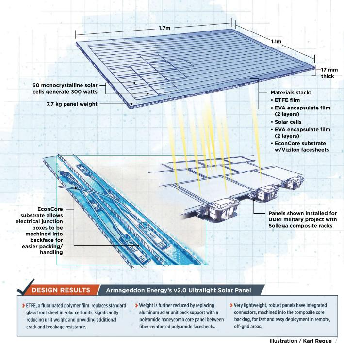
"We wanted to move beyond glass, and with ETFE films, our first version was light enough for a child to lift with one hand, and unique in design," says Goldman. "The pre-wired, rapid-assembly racks were designed for installation by a roofer or electrician, with no special solar training." One notable rooftop installation of SolarClover is the City Hall in San Jose, CA, US.
