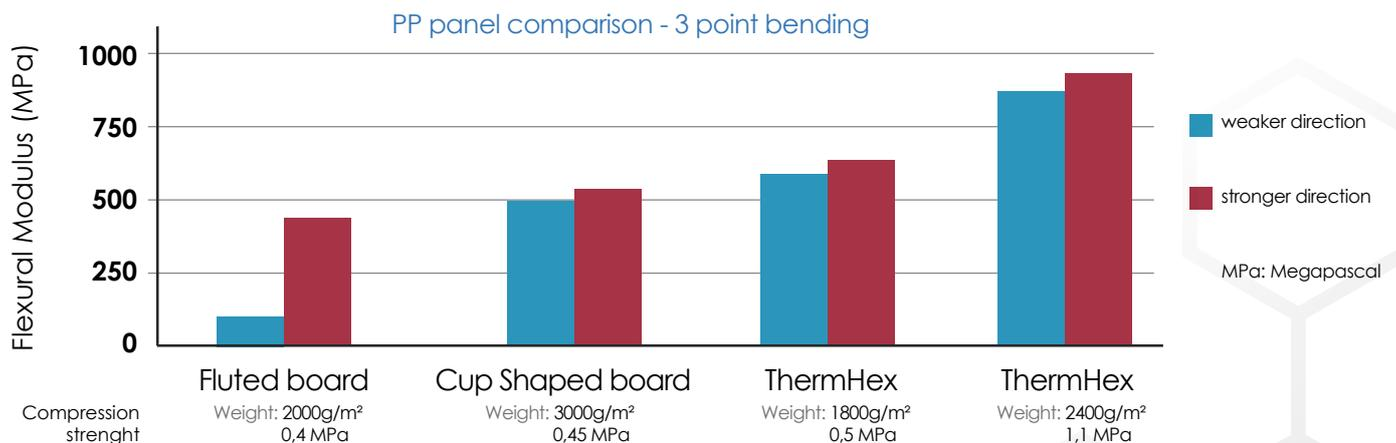
The 3 point bending measurements demonstrate that the ThermHex based panels outperform the traditional fluted and cup shaped base panels on stiffness. The ThermHex performance is even more remarkable if one realizes the significant weight reduction of these ThermHex panels versus the traditional products.
