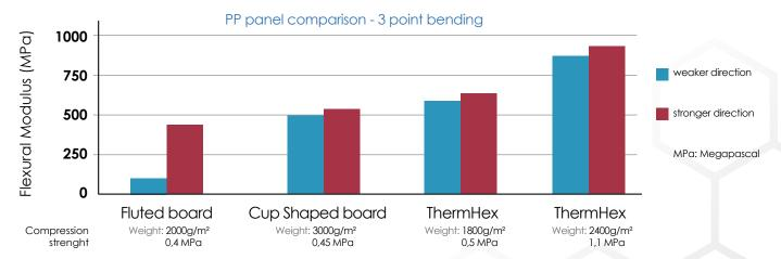
The 3 point bending measurements demonstrate that the ThermHex based panels outperform the traditional fluted and cup shaped base panels on stiffness. The ThermHex performance is even more remarkable if one realizes the significant weight reduction of these ThermHex panels versus the traditional products.
